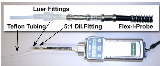
Figure 4. Connection to a PID with Flex-I-Probe.
