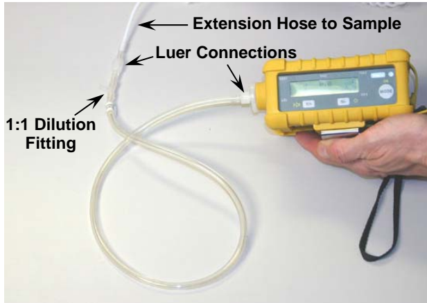
Figure 3. Connection to an instrument with Luer fittings. Keep the dilution fitting away from the gas outlet port, to ensure clean air is used for dilution.
