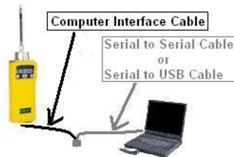
Figure 8. Hardwiring RAE Wireless Detectors.
